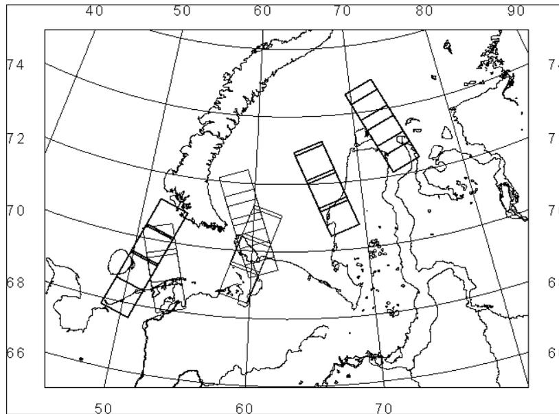
*Figure 2. In the NERSC database for March 1994 are 137 ERS-1 SAR images for the Kara and Pechora Sea area. The good coverage and many near-coincident scenes are due to the satellite's 3 day repeat 'Ice orbit' in January-March 1994. This makes it possible to compute ice displacement at different locations throughout the month.*
